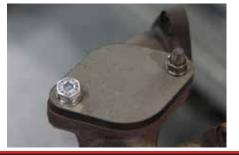
**2007.5 -2012 Only** Add a little assembly lube onto coolant plug and install. Add tear drop style bracket onto the coolant line as shown, and attach support bracket from cylinder head to the coolant plug.
