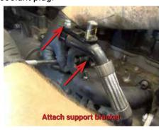
**2013 -2016 Only** Install supplied coolant distribution pipe and o-ring into the coolant inlet housing on the block, re-using factory hardware.
