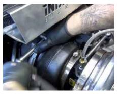
Install the supplied turbine blanket onto the large charger. Make sure there is enough room for the blanket to slide between the turbine housing on the large charger and the compressor cover on the S300. Use the supplied metal zip ties to secure the turbine blanket through the eyelets. Do not overtighten. Cut off the excess zip tie when finished.
