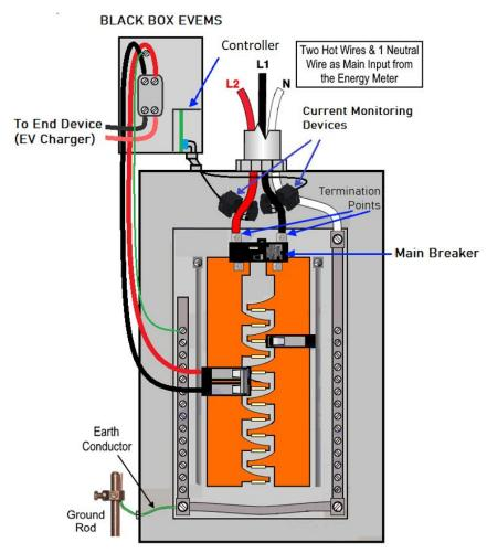
Alternate locations for devices installation are acceptable
