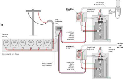
\*This device does not need additional breakers to what is required to feed the 240-208VAC end device to be controlled. The service size and end device current is to be set by the installer. See installation manual. Designed and manufactured in Canada. Inspected and labeled by Intertek in Canada.
