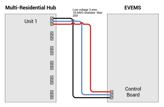
Incorrect wire orientation will cause system not to function, and could cause damage to the energy management installation.
