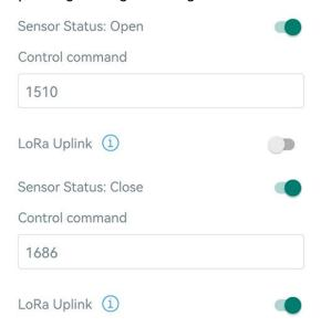
**Note:** If you enable **LoRa Uplink** feature, LoRaWAN® uplink packet that contains the sensor's magnet status will be sent to gateway after the Milesight D2D control command is sent.
