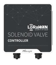
IOT-C51x series LoRaWAN® Solenoid Valve Controller is a device used to remotely control DC latching solenoids of the valve. It contains 2 solenoid interfaces and 2 GPIO interfaces, which can be easily controlled locally or remotely.
