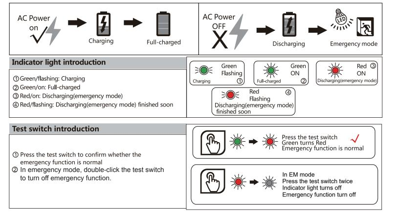
\* Note: AC power on, click the test switch, switch to emergency mode and lasts 3S, then automatically back to the working mode of AC power supply
