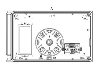
A - 1/2" NPS tapped holes (surface conduit or photo contro I)
