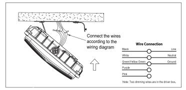
2. Fix the mounting plate to the ceiling with the screws.
