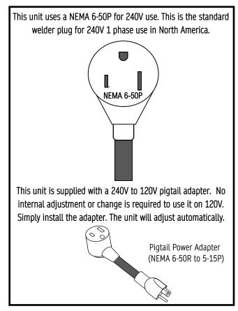
**CAUTION:** Use only with extension cords 50 feet long or less, rated for 240V welder 50A use, or damage may result. For 120 operation, use only with 30A rated cords, less than 25 feet in length.
