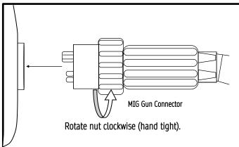
**IMPORTANT!** Remove MIG Gun while using Stick process. The MIG Gun will remain live if connected. If it comes into contact with metal, the MIG Gun may short out, and may cause damage to the unit. Personal injury may also occur.
