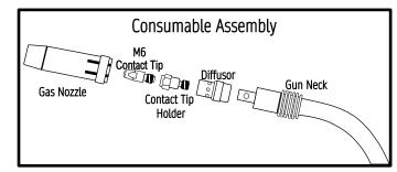
Hold the gun cable and gun straight as possible. Press and hold the cold feed wire button on the panel. The wire should slowly begin to feed through the gun cable and eventually through the gun. As the wire exits the gun, allow 3 to 4 extra inches of wire to be fed out past the diffusor. Re-install the contact tip over the wire and screw it in clockwise until it is tight. Be careful not to strip the threads. Install the gas nozzle. Trim the wire before welding. See the illustration below.
