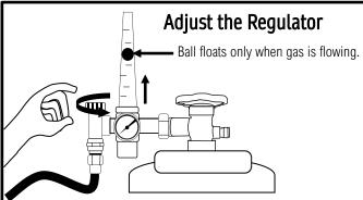
Turning the adjustment knob counterclockwise (when viewed from the top) increases flow rate. Turning the knob clockwise until it seats will shut off gas flow at the regulator. Do not use the regulator to shut off the gas flow. Shut off the gas flow at the cylinder when the welder is not in use for more than 20 minutes.
