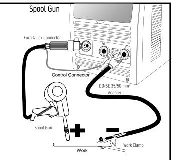
The spool gun connection process is similar to the MIG torch connection and uses the same Euro Quick Connect connection. Polarity configuration is the same as MIG except when Flux-Cored wire is being used. If Flux-Cored wire is being used, then use the standard Flux-Cored polarity.
