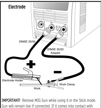
Gun will remain live if connected. If it comes into contact with metal, the MIG Gun may short out, and may cause damage to the unit. Personal injury may also occur.
