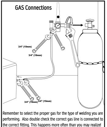
seal the threads. If the threads do not seal, remove and check the connections for debris or pieces of metal on the sealing surfaces.
