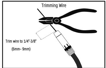
The unit comes with and .035" and .045" drive rolls installed. NO-TICE: *For most purposes you will likely want to use .035" wire in this unit since it covers the greatest range of metal thicknesses and amperages within the capability of this unit.* However, if you change wire size or type, you will need to change the drive roll to the correct size and type. There are extra sizes and types in the bag for the consumables.
