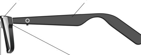
To tighten or loosen temples significantly, heat the bridge and bend it inward or outward slightly.
