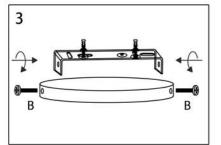
3. Please Place the suction top plate on the hanging plate and then screw the nut B into the hanging plate to fix the suction top plate.
