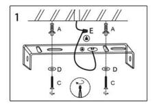
2. Please use terminals E to connect the N pole and L pole to the power wire correspondingly. 1. Please drive the expansion bolts A into the ceiling wall, put the discs D into the self-tapping screws C. pass through the hanging plate, and then screw the self-tapping screws C into the expansion bolts A to fix the hanging plate on the ceiling. Please use terminals E to connect the ground wire.
