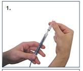
1. Invert the electrode. Hold the electrode just below the sleeve and with careful rotation and pulling along the axis of the electrode, remove the sleeve. DO NOT BEND.
