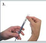
3. Slide the sleeve back onto the electrode ensuring the black O-ring is well seated within the electrode body. Do not exert sideways force. Any excess electrolyte will be expelled from the end of the electrode through the ground junction. Ensure there are no air bubbles in the sleeve.
