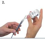
2. Fill the annular space with gel or electrolyte to approximately half-to three-quarters full.
