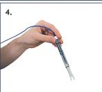
4. With the pH bulb facing downwards, gently flick the electrode to remove any bubbles from within the membrane. Wash off any excess electrolyte and store in 2-3M KCl before use.
