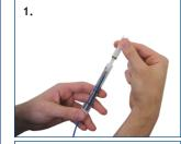
1. Invert the electrode. Hold the electrode just below the sleeve and with careful rotation and pulling along the axis of the electrode, remove the sleeve. DO NOT BEND.
