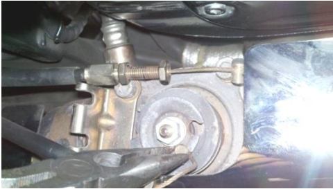
Fig. 1.4 remove barrel cables
