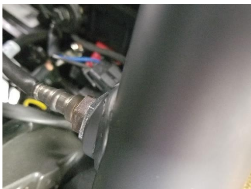
Figure 2.7 install front oxygen sensor
