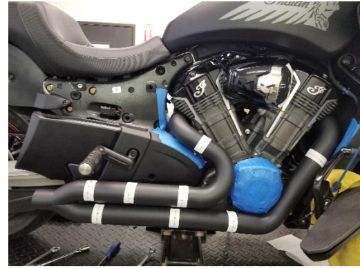
Figure 2.12 place rear shield over pipe
