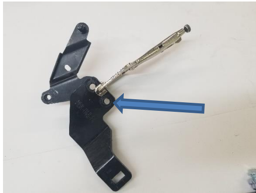
Figure 2.1 place new bracket on top of stock bracket and mark the center
