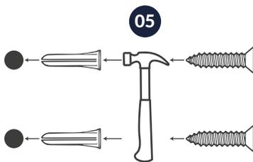
5. Place the 2 plastic anchors in the holes and push them with the help of a lite hammer.
