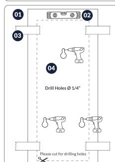
Once the location for the Soap dispenser has been decided, proceed with the installation steps below. If the soap dispenser is installed above the sink, leave a space of 18" from the top of the sink to the soap dispenser as shown below in figure (A).
