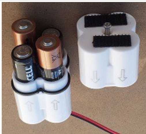
Open cap and replace with Duracell brand copper top batteries only. Make sure to insert batteries as shown in photo.
