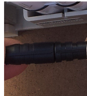
Make sure that pins line up with receptacle holes, then line up stripes as shown in photos above prior to inserting plugs.
