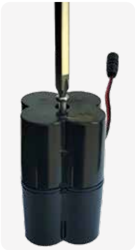
When reinstalling cap, align arrows and tighten screw using #2 Philips screw Driver.
