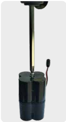
Remove Screw using a #2 Philips screw driver.
