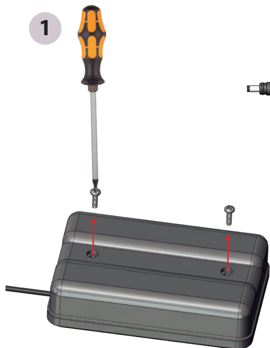
Unfasten 2 cover screws, and lift cover up and away from batteries
