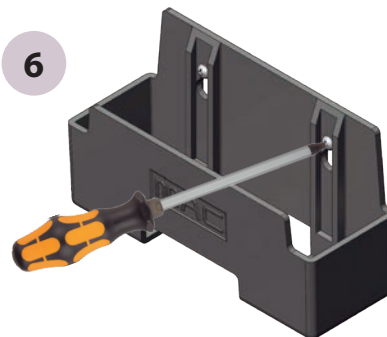
Install Battery case holder onto wall in a level horizontal position.
