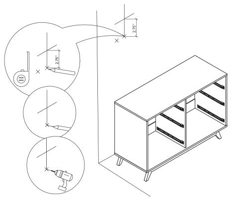
Drill four holes at the pencil marks on the wall with a diameter of 5/16 inch (8mm)
