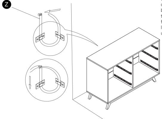
Move the dresser to its final position. Lace one end of the restraint strap through the larger hole on each mounting bracket. Bring both ends together and slide the flat end through the locking end. Pull through until all slack is removed.
