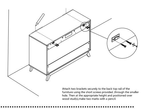
Drill two 5/16 inch(8mm) diameter holes through the wall at the height you marked with pencil
