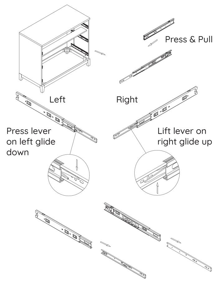
The silver portion of the glide must be pulled to the front of the glide when assembling the drawer into the case.
