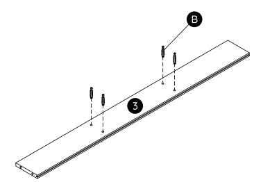
• Rotate 'B' clockwise to secure.
