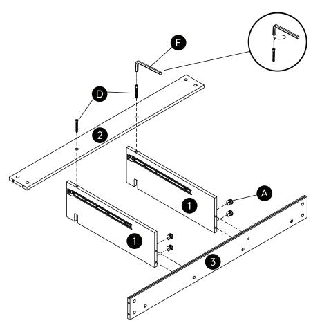
• Rotate 'A' clockwise to secure, Tighten 'D' clockwise with 'E'.
