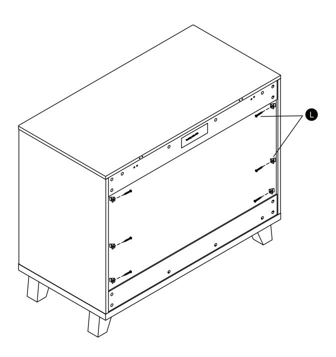
Put the plastic bracket insert if necessary
