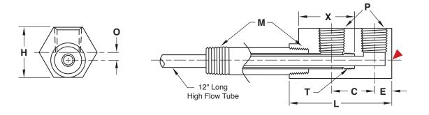
M Head: Brass, Tube: Stainless Steel, 2" Long Pipe Nipple: Stainless Steel
