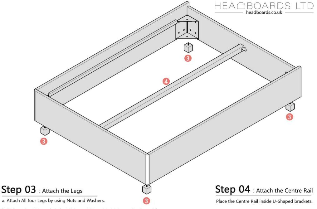
b. Tighten the All Loosely Bolted Fixings of ( Step 1 & 2 ) Corner Brackets with Side Rails and Cross Rails as frame is settled now in gravitational force.
