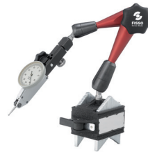
S-20.30 with anyform magnet (AM) (permanent)
