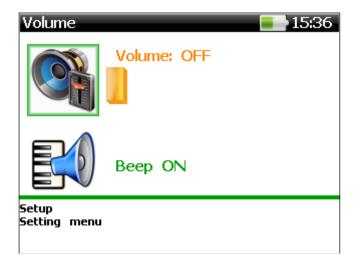
Select the desired function (Speaker Volume or Key Beep), using the up and down arrow keys. Change the current value using the left and right arrow keys. Save the new value using the ENTER key or discard the changes using the ESC key.
