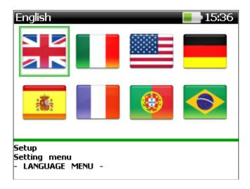
Select the desired language using the arrow keys and save the new selection with ENTER or discard the change using the ESC key.
