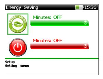
Select the desired function (Energy saving and Switching OFF delays), using the up and down arrow keys. Change the current value, using the left and right arrow keys. Save the new value, using the ENTER key or discard the changes, using the ESC key. To disable the Energy saving and/or Switching OFF delays, press the left arrow key repeatedly until the OFF message appears.
