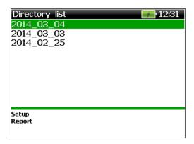
Screenshots are stored in the internal SD memory folders labelled with the date format YYYY\_MM\_DD. The label indicates the date of the image creation. In each folder, the images are saved using bmp format. The file name contains date and time of creation, according to the standard YYYY\_MM\_DD-HH\_MM\_SS.bmp. After selecting the desired folder, the following screen appears:
