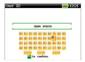
Navigate the virtual keyboard with the arrow keys, select the single characters with ENTER and confirm the text entered using the F3 key.
