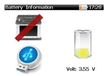
The previous screen displays on the left side the current power source: motorcycle battery, USB or none. The device battery current voltage and the residual charge are displayed on the left side of the screen. When the device is connected to a vehicle, the power source is the 12V battery and the battery screen changes as follows:
