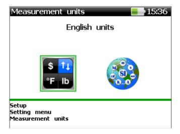
Select the desired measurement units using the left and right arrow keys. Save the new value, using the ENTER key or discard the change, using the ESC key.
