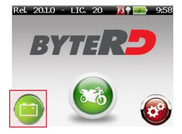
Select the Battery information icon (battery logo) using the left and right arrow keys and confirm with ENTER
