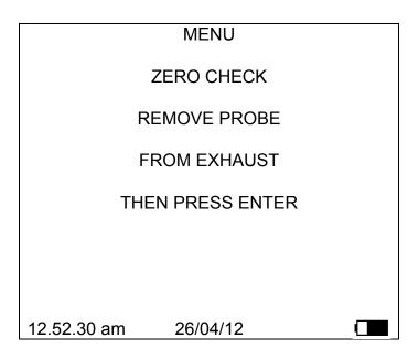
Ensure the probe is removed from the vehicle exhaust and is sampling fresh air, in the garage environment this should be ½ meter or 18 inches above the ground. Once this is done press to activate the pump.
