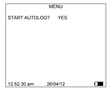
To initiate AUTOLOG go back to the main display where the Autolog time will be displayed in the top right hand corner of the display, and then press . The analyzer will beep and the autolog time will disappear for a second or so.
