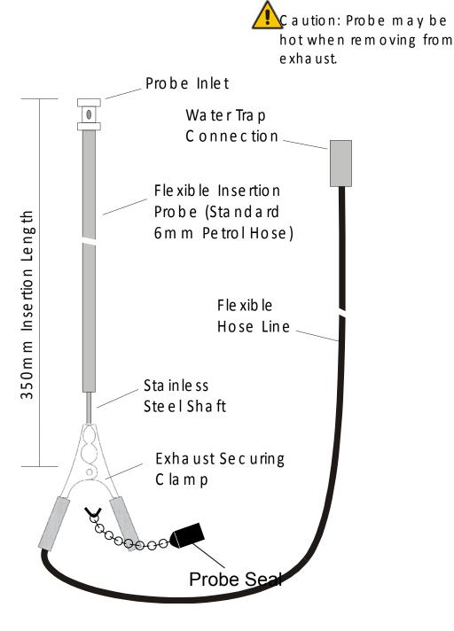
**Note:** A variety of probes are available, including high temperature probes necessary for on-road / rolling road vehicle testing when the temperature of the emission gases increase. Please request further details from your distributor or contact Kane International Ltd directly.
