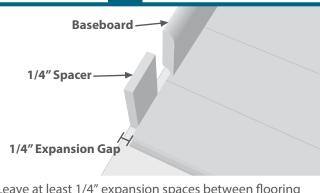
Leave at least 1/4" expansion spaces between flooring and ALL vertical objects (walls, cabinets, pipes, etc.) Large flooring runs may require additional expansion space. Undercut door jambs and casings to provide adequate expansion space. Cali Bamboo® does not recommend screwing or nailing cabinetry or other permanent fixtures to the flooring.
