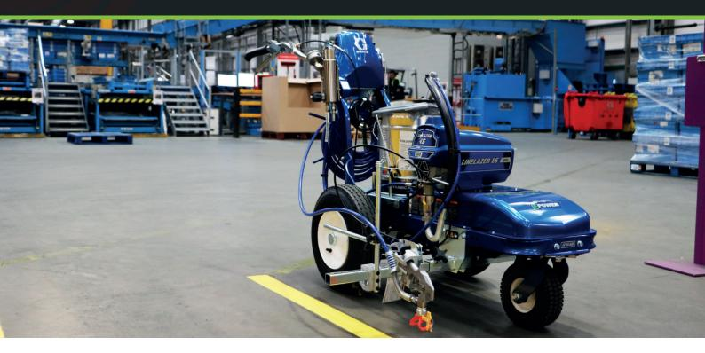
The LineLazer ES 1000 is an electric airless line marking machine powered by a high-output lithium battery – allowing it to be used safely indoors and outdoors while having the power and performance needed for all jobs. "Go Green" with this quiet, fume-free machine! No engine noise, no engine vibration and no engine fumes!
