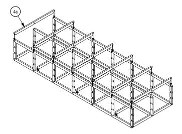
From the front and bottom of the rack, firmly apply pressure to lock the joint. Then apply two nails with a nail-gun, to each joint. Remember to firmly lock in each joint.
