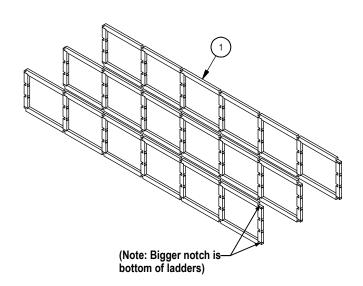
From the bottom and working your way up, place the back spacer bars (4b) according to the ladder notches. Make sure to carefully interlock the spacer bars to the ladders.
