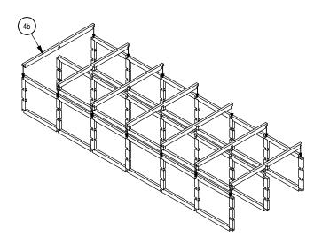
Once the spacer bars are properly placed. Start from the bottom of the rack, firmly apply pressure to lock the joint. Then apply two nails with a nail-gun, to each joint. Remember to firmly lock in each joint.
