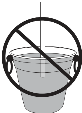
WRONG: Drain line is under water.
