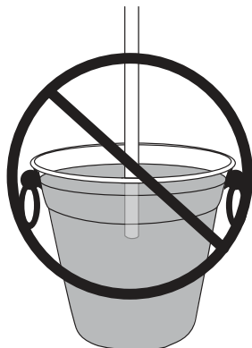
WRONG: Drain line is under water.
