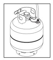
3. Apply the soap solution to the gas connections using a soft bristle brush.
