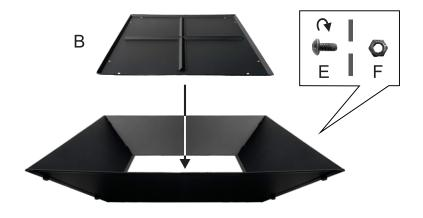
Step 3: Assemble the fence front and sides with the bots and nuts.
