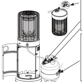
Soap bubbles will appear if there is a gas leak. In case of a leak, turn off the gas supply. Tighen any leaking fittings, then turn the gas supply on and re-check.
