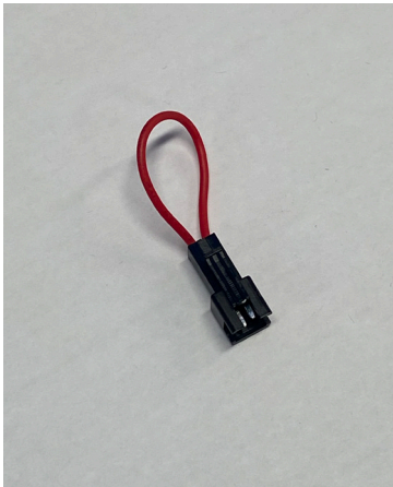
Figure 5: Red Jumper Wires
