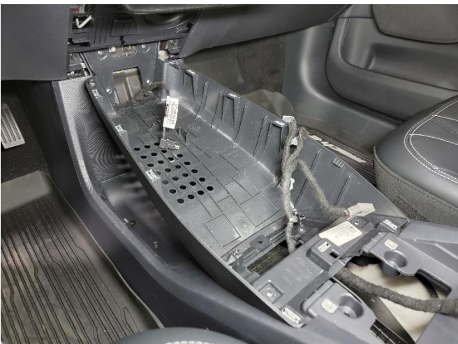
Remove all remaining modules and harness from lower center storage area
