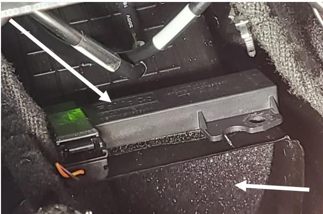
Position and attach front OEM Key sensor side to side inside console on top of air duct with 10-32 x 1/2" screw and nut. Drilling plastic dust required. Insert foam into vent to prevent air from blowing inside console.
