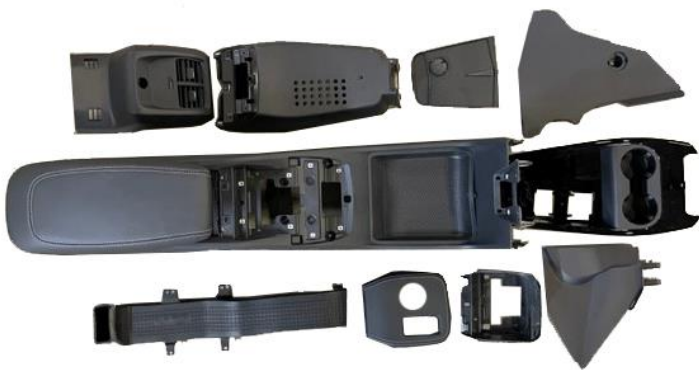
Remove all OEM center console parts. Save hardware for possible future use.
