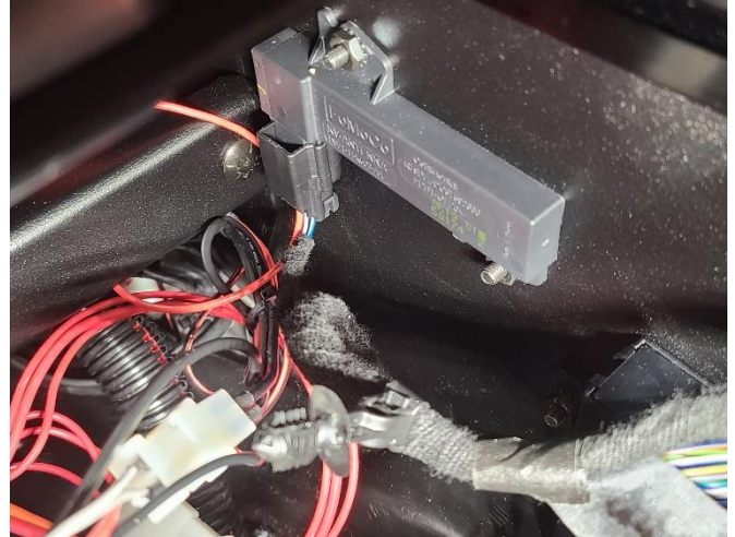
Attach Rear OEM Key sensor inside console housing with 10-32 x 1/2" screw and nut and plug in wiring.
