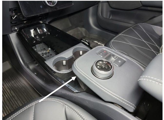
Remove shifter and emergency brake pad by gently pulling up from the front.
