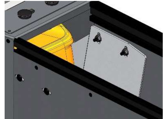
Loosely attach housing to brackets with 1/4" x 3/4" carriage bolts and serrated nuts. Double check positioning.
