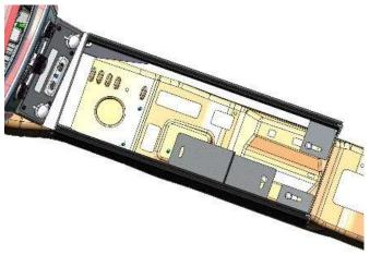
Cover (11209) is provided to guard the OEM sensor on the transmission hump. Attach cover using  $\frac{1}{4}$  x  $\frac{3}{4}$ " self-threading screw.
