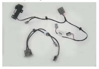
Remove sensor and 12 volt socket wire harness assembly from under side of OEM console.
