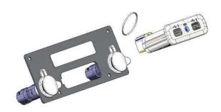
Place supplied rubber "O" ring onto the OEM module.
