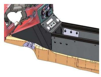
Attach trim panels using #8 x 3/8" supplied screws.
