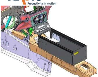
Slide main console housing onto floor bracket. Plug OEM wire harness back onto original connectors and into repositioned OEM equipment.
