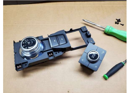
Carefully unsnap the Drive mode switch from the bezel.
