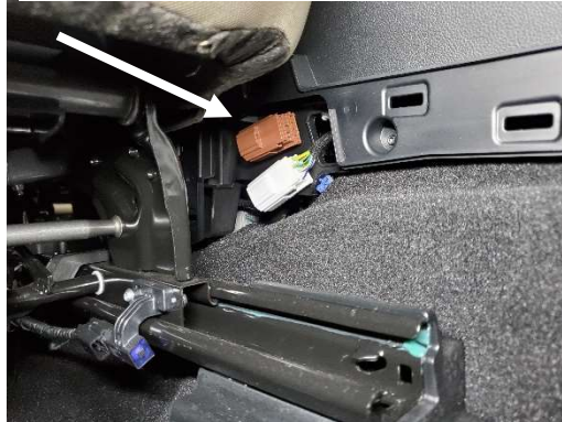
Disconnect (2) plugs from both middle sides of OEM console. (Driver side not shown)
