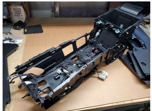
Remove side panels from OEM console and remove harness. Harness will need to be re-installed into vehicle.
