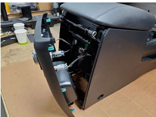
Remove OEM rear end panel and disconnect all plugs.
