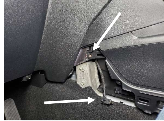
Unsnap OEM console lower trim on driver and passenger sides. Remove (1) bolt each side from forward end of the console. (7mm socket) Unplug USB on driver side
