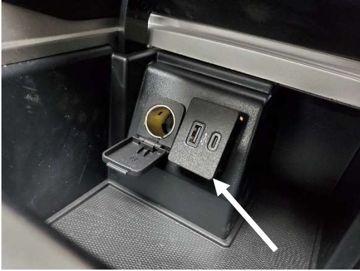
Remove OEM aux panel and 12v socket from forward section of OEM console.
