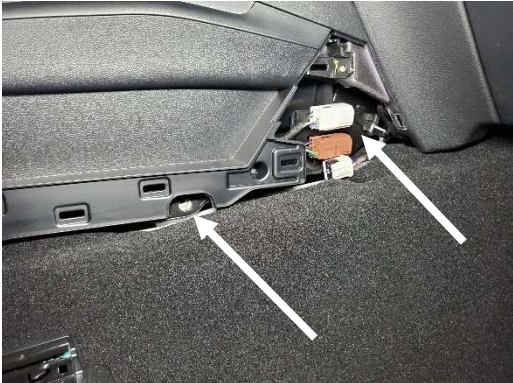
Remove (1) bolt each side from side of console. (10mm socket) Disconnect (2) plugs at front passenger side of console.
