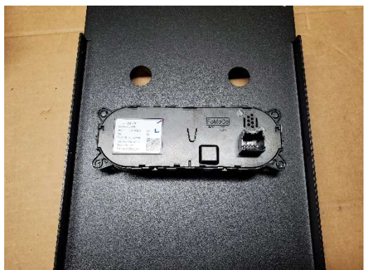
Relocate OEM 12v sockets and rear HVAC control to new end panel. Attach control with supplied 10-32 x 1/2" screws and flat washers.
