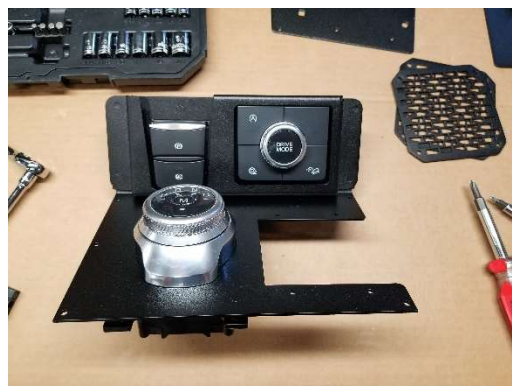
Install previously removed parts into new shifter plate using supplied 10-32 x 1/2" Phillips machine screws.
