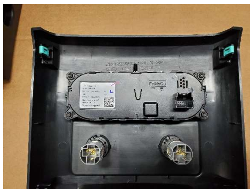
Remove rear 12v sockets and rear HVAC control from OEM console end panel.
