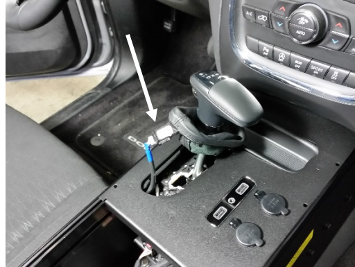
Carefully place top faceplate onto console and attach with # 8 x 3/8" Torx head screws. Slide shifter back on and plug in shifter boot to OEM harness
