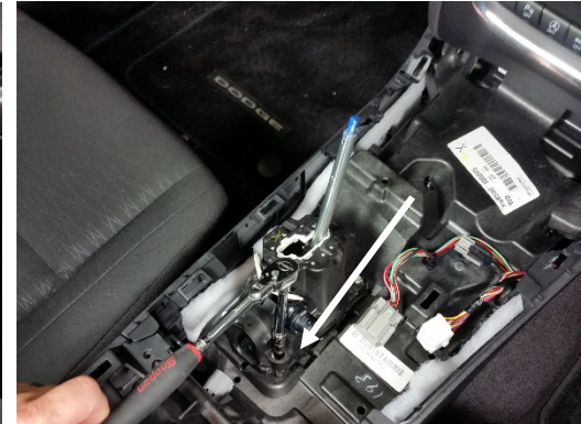
Unbolt shifter assembly from center console using 8mm socket and ratchet.
