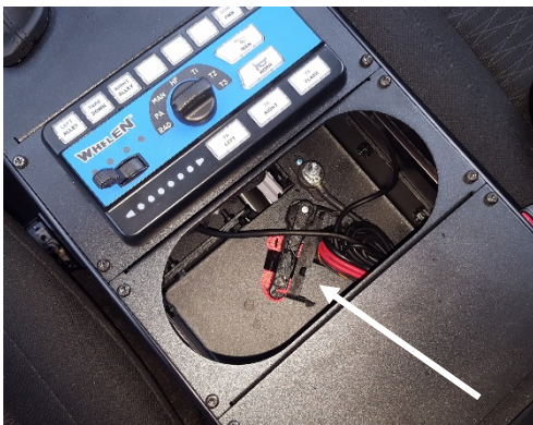
Manual park release needs to be looped inside console and located so access can be done by removing cup holder.
