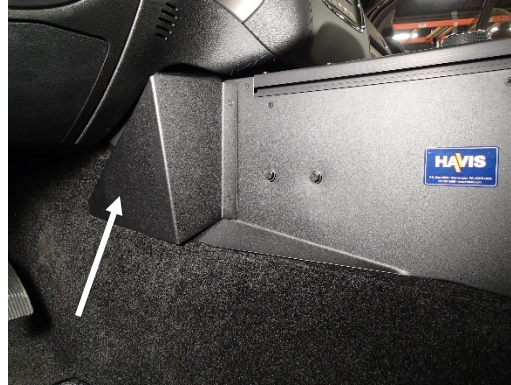
Attach driver side trim panel to console housing with # 8 x 1/4" flat head sheet metal screws.
