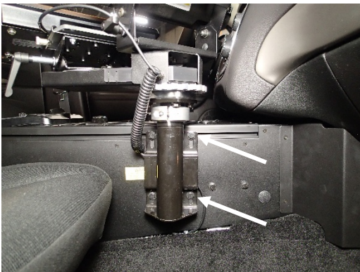
If mounting a C-HDM-204 or 214 side computer mount, use the existing 1/4" hex nuts with 1/2" hex bolts and flat washers in upper side extrusion. Use 1/4" x 3/4" hex head bolts and flat washers for bottom mounting.
