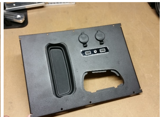
New console faceplate ready to be installed. Note: Some vehicles will have the coin tray/traction control knob that mounts the same way.
