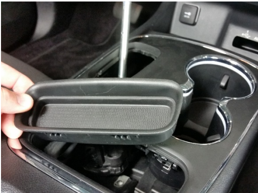
Carefully pop out coin tray from console top panel. (coin tray to be reused) Note: Some vehicles may have a coin tray/traction control switch.
