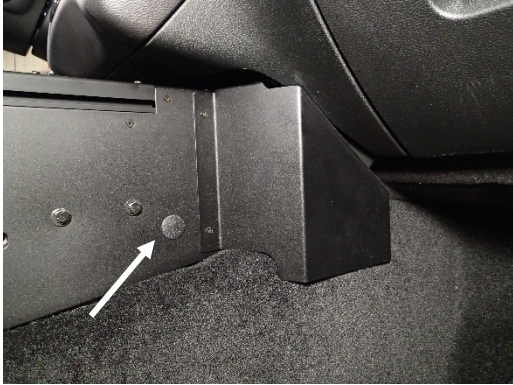
Attach passenger side trim panel to console housing with # 8 x 1/4" flat head sheet metal screws. This photo also shows the alternate location for the 12 volt socket.
