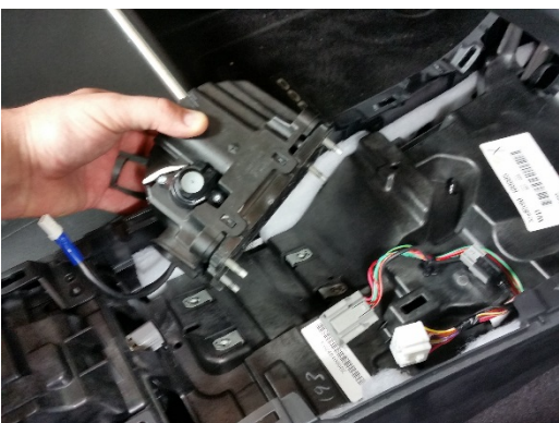
Unplug and remove shifter and set aside. (OEM bolts will not be reused)
