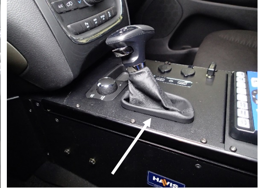
Tighten Allen head bolt to OEM shifter stalk. (9/64" Allen wrench) Snap shifter boot down into shifter boot plate
