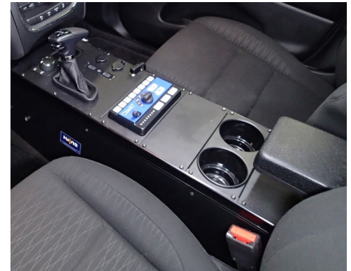
Run wiring as needed. Mount face plates and accessories into console with # 8 x 3/8" Torx head screws. Screws supplied with equipment brackets and accessories.
