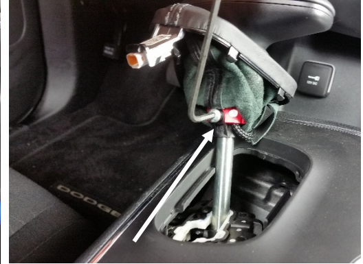
Loosen Allen head bolt and remove shifter handle from stalk. (9/64" Allen wrench)
