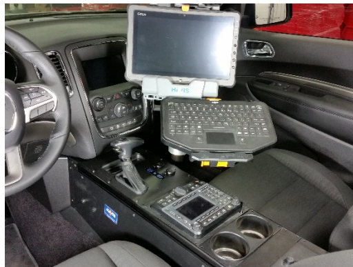
Install computer mount assembly and make final adjustments.
