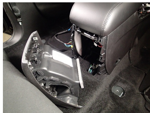
Carefully unclip and remove rear console end panel. Unplug wires as needed. Some vehicle may not have wiring.
