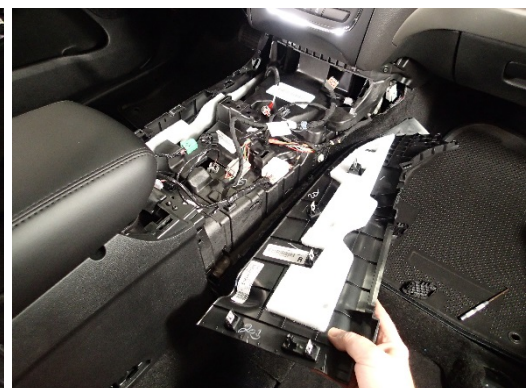
Carefully unclip and remove console forward side panels.
