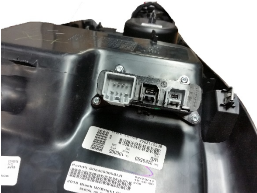
Remove forward Aux input module. (T-20 Torx)
