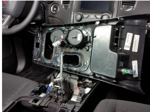
Carefully unclip and remove top console panel. Unplug all wire connectors.
