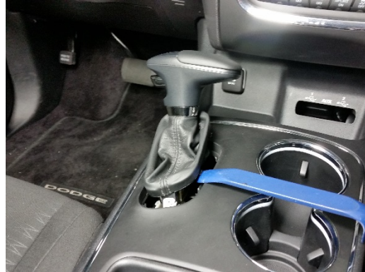
Carefully pop up shifter boot and unplug sensor from rear of boot.
