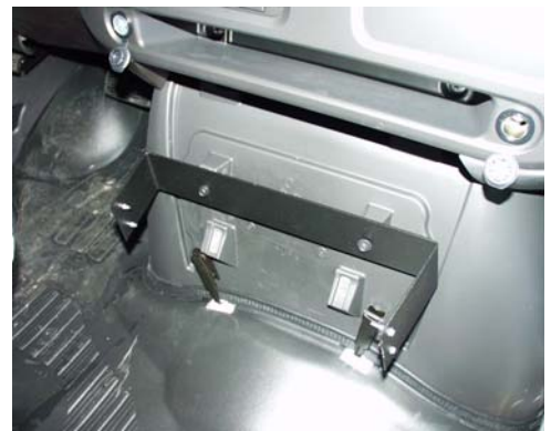
Attach vehicle-mounting bracket using OEM hardware
