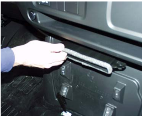
Make sure blower duct remains in place
