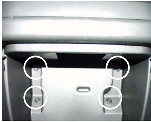
Remove (4) 10mm bolts from inside lower OEM console pocket
