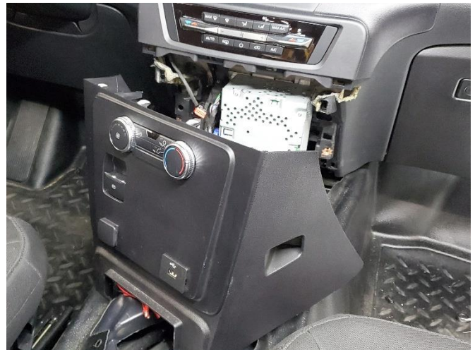
Remove lower dash trim by carefully pulling it towards the rear of the vehicle.
