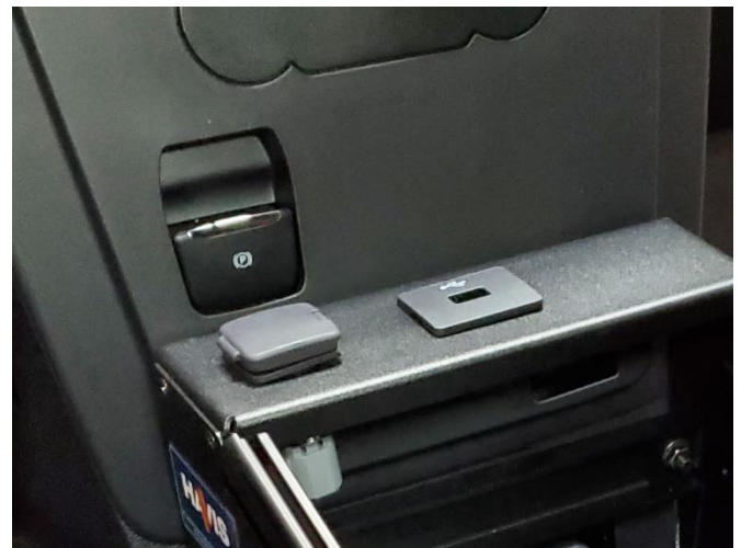
Install OEM 12 v socket and USB retaining bracket into console top forward panel.
