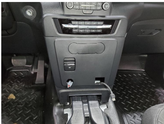
Unplug and remove OEM 12 v socket and USB module. Re-install lower trim and OEM fasteners into dash.
