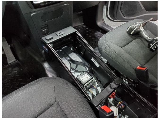
Slide console housing onto floor brackets and attach with carriage bolts and serrated nuts. Tighten all hardware.
