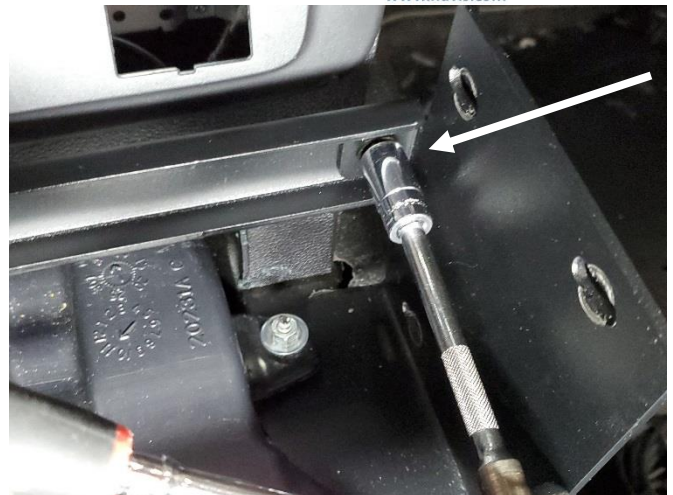
Attach front lower cross support to mount brackets with carriage bolts and serrated nuts.
