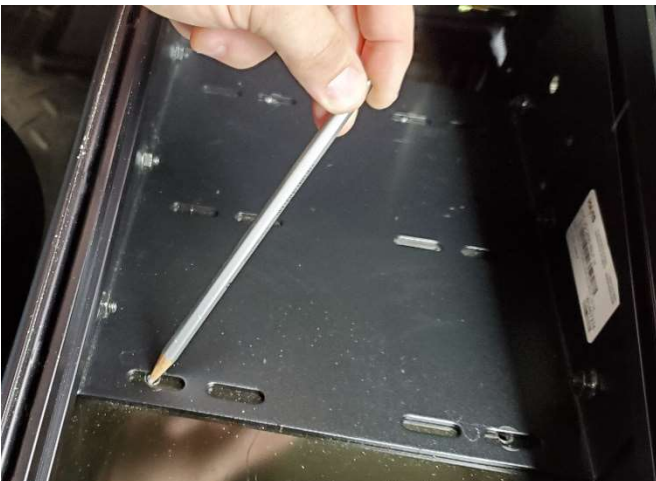
Mark the tunnel plate using a pencil or marker.
