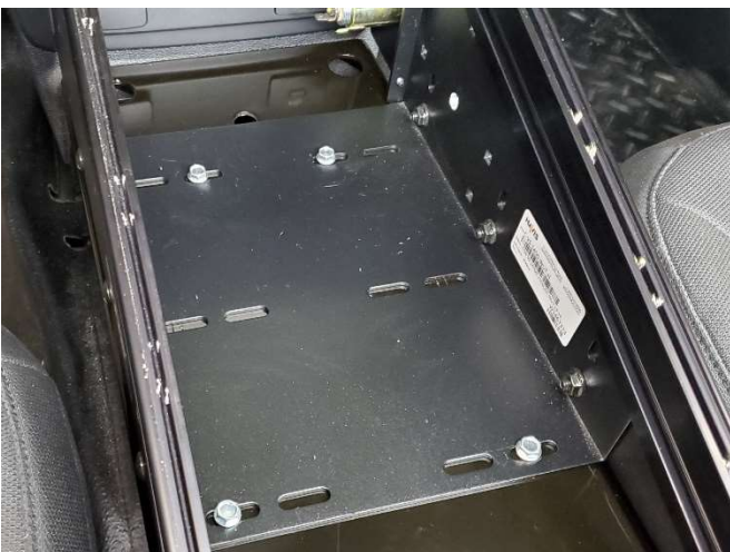
Reinstall console and attach using four (4) 1/4" x 3/4" self-threading bolts.
