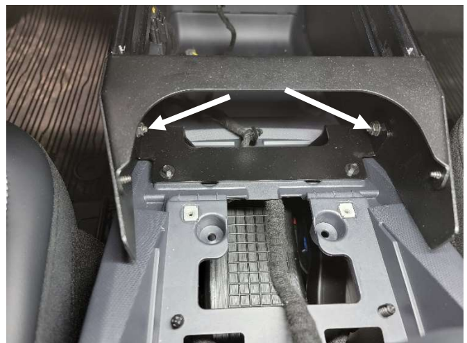
Place console over mounting brackets and attach to the rear bracket using 1/4" x 3/4" carriage bolts and serrated nuts.
