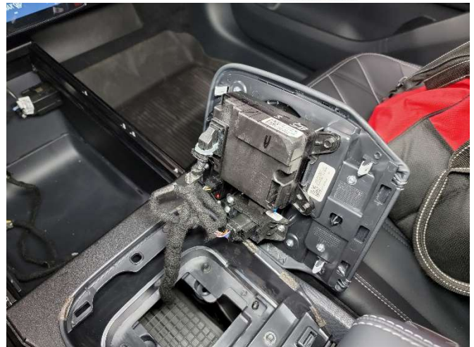
Plug in shifter and emergency brake. Snap shifter plate back into the center console.
