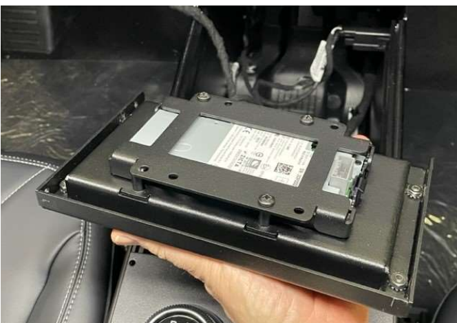
Place OEM wireless charger into rear of charger faceplate and bracket. Attach adaptor bracket with 10-32 x 1/2" screws to hold charger in. Install assembly into console.
