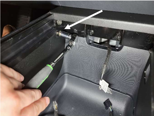
Attach to the front bracket using 1/4" x 3/4" carriage bolts and serrated nuts.
