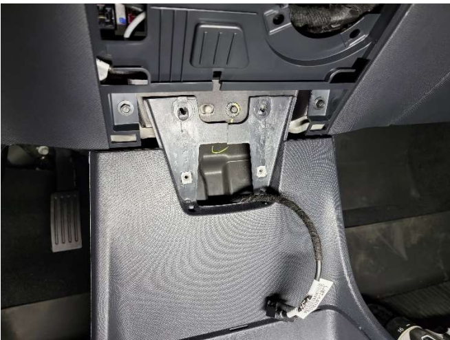
Remove lower, center storage area.
