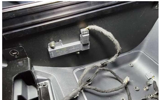
Install key sense module on side of console using supplied #10 hardware. Double check keyless function after everything is installed. Relocation of sensor to central forward location may be required for proper reception.
