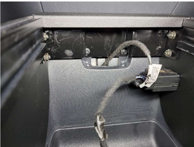
Install previously removed AUX panel into side of console and plug in.
