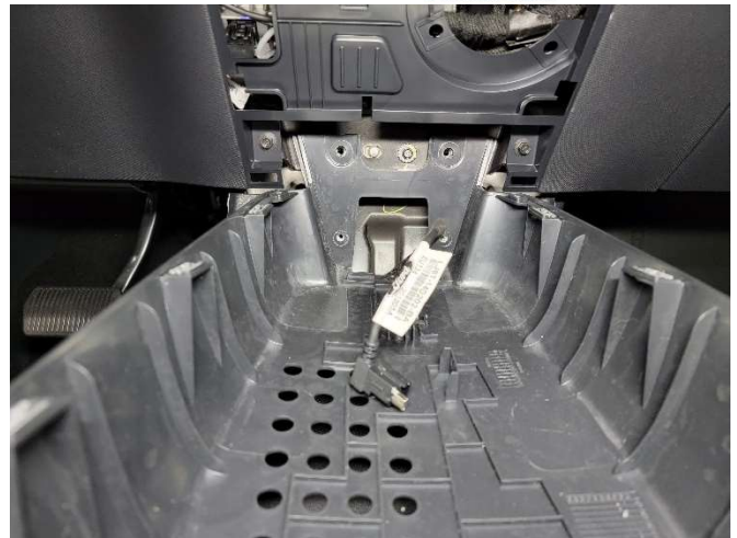
Unsnap trim from upper section or lower, center storage area and remove (4) OEM fasteners.
