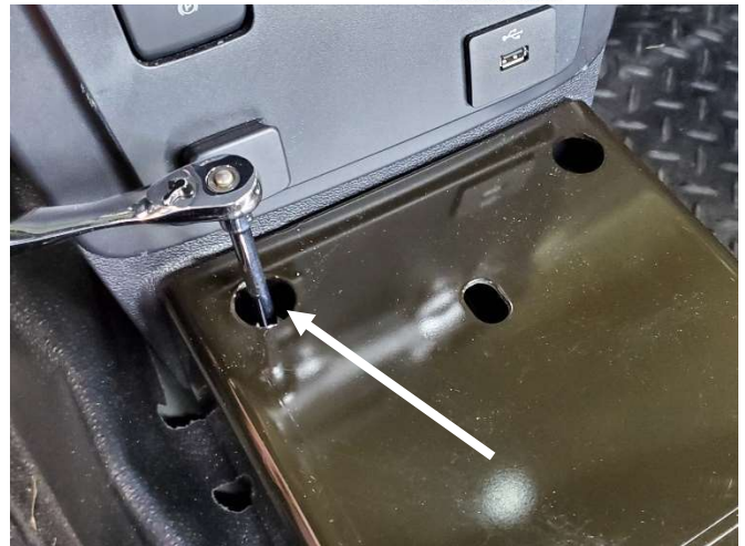
Remove OEM tunnel plate by removing rear nuts. Front nuts only have to be loosened. The OEM track is slotted at the front. (10mm socket)
