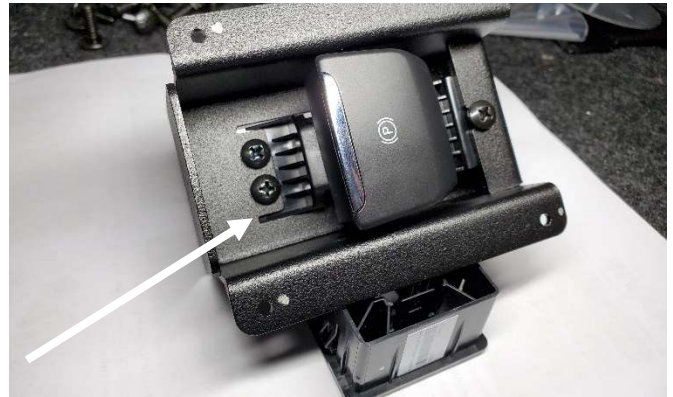
Attach switch to bracket using (3) 10-32 x 3/4" screws and Keps nuts.
