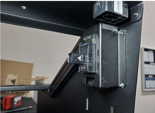
Attach brake switch bracket to console using (4) #8 x 1/4" flat head screws.
