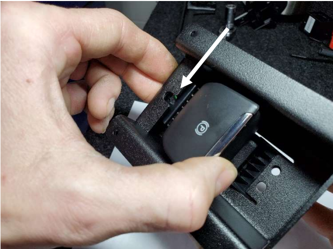
While pushing the brake switch forward, slide the rear of the switch under the lip of the bracket and lineup the holes.
