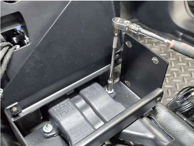
Retighten OEM ductwork nuts and bracket hardware.
