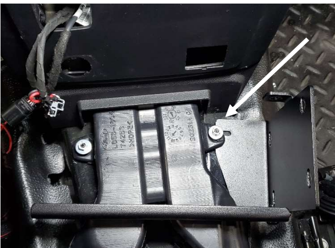
Loosen OEM nuts from front ductwork. (10mm socket) Slide front mounting brackets under ductwork from the sides onto OEM studs. Note: Make sure brackets are below plastic vent and sitting on top of metal floor.
