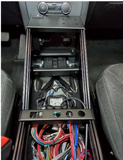
Place console over previously installed brackets and attach with carriage bolts and serrated nuts. Ensure console is tight to dash. Tighten all hardware.
