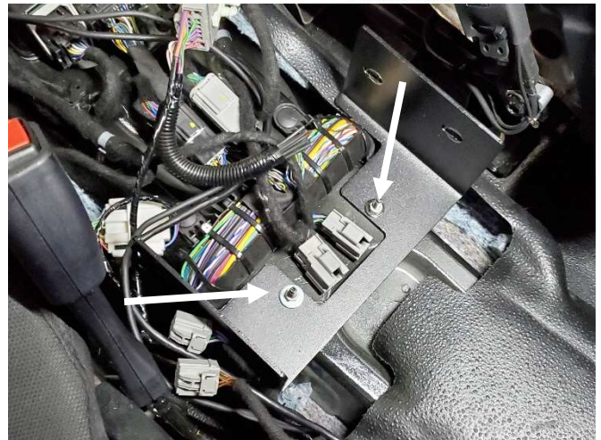
Attach rear mounting bracket to floor studs using previously removed OEM nuts. (10mm socket)
