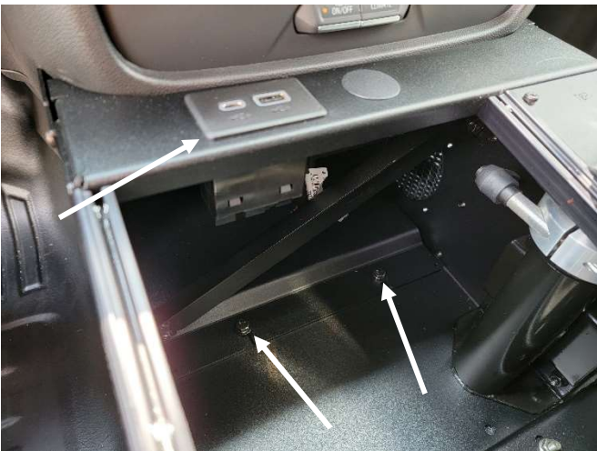
Loosely attach tray to support bracket using (2) 1/4" x 1/2" bolts, split lock washers, and flat washers.
