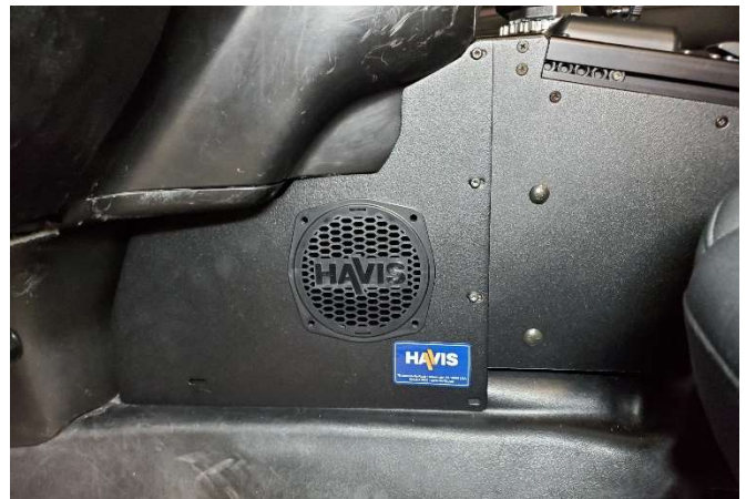
Attach forward side filler panels to console and equipment mounting tray using #8 x 3/8" Torx screws. Tighten all mount hardware. Install OEM 120 volt socket into passenger side panel.
