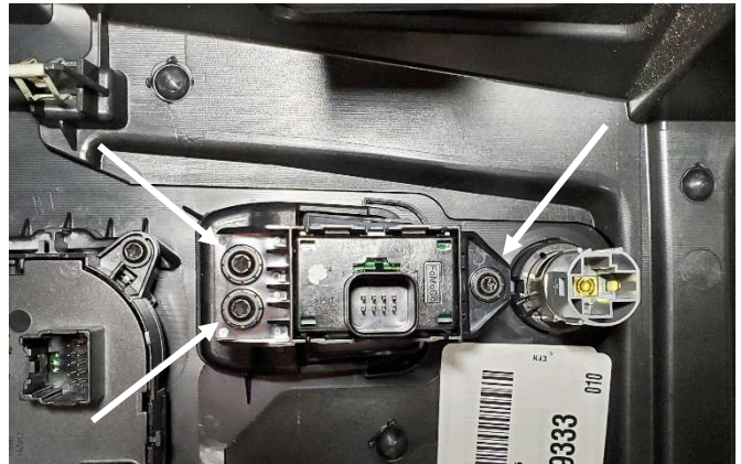
Remove electronic parking brake, 12 v socket and USB retaining bracket. (T-20 fasteners) If vehicle is equipped with rear HVAC, the controller will be removed at this time. Re-install trim with OEM fasteners back into dash.
