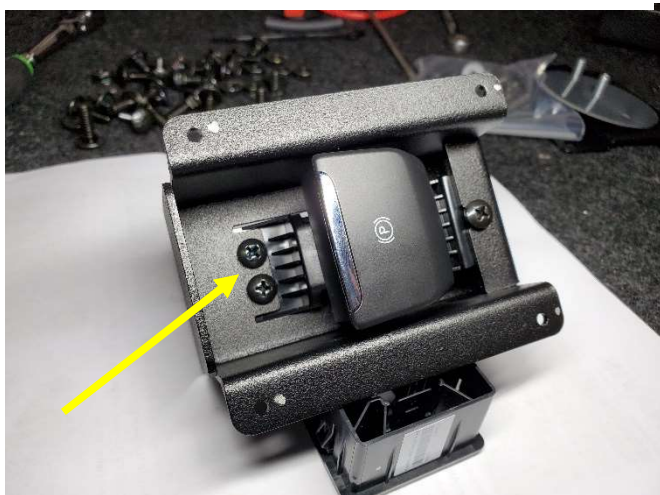
Install previously removed parking brake switch into supplied relocation bracket. The angled section with two holes goes under the lip of the bracket. Attach with (3) 10-32 x 3/4" screws and Keps nuts.
