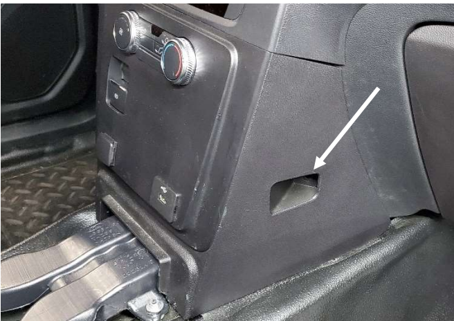
Remove fasteners on sides of lower center trim and detach from dash by pulling it towards the rear of the vehicle. (7mm)
