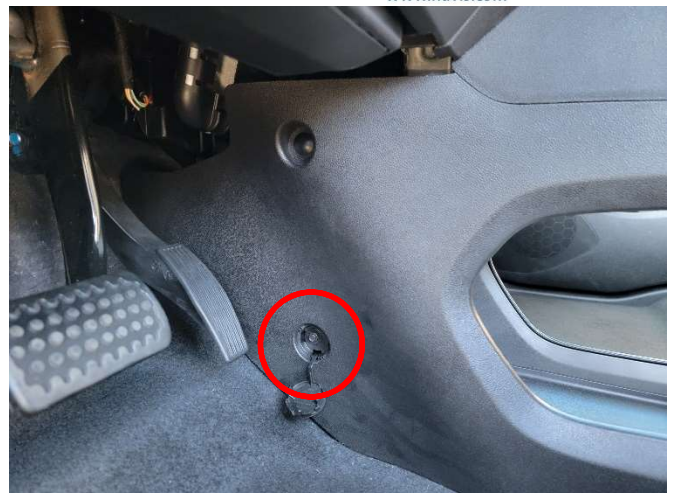
Remove cover and plug from lower driver and passenger side panel. Unbolt the 10mm OEM fastener and set aside.
