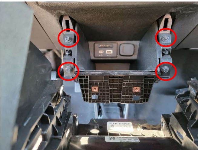
Remove the (4) OEM equipment tray bolts shown.
