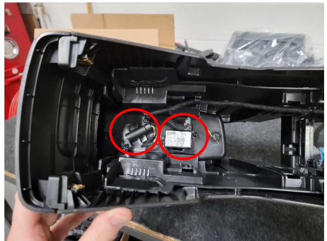
Remove OEM modules from under side of OEM console
