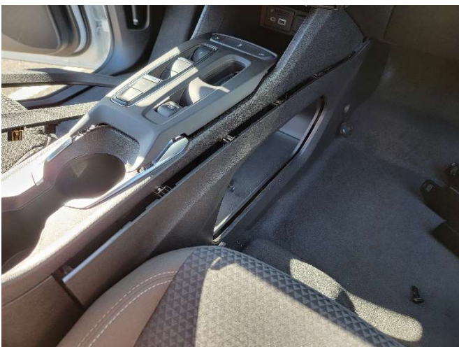
Unclip and remove both driver and passenger side panels.
