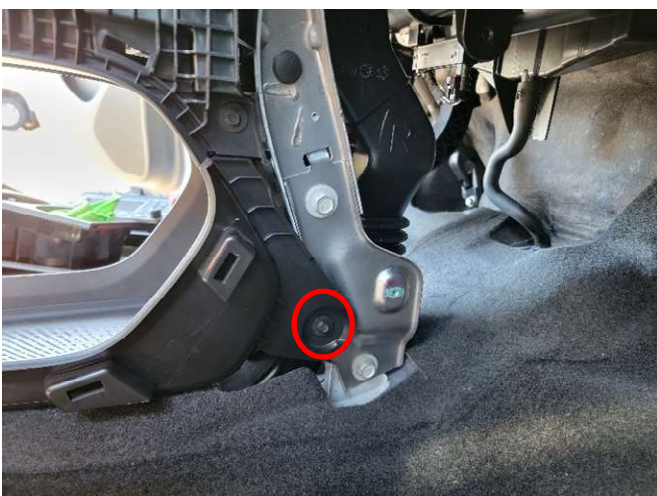
Unbolt the (2) 10mm OEM fasteners on the exposed plastic structure and set aside
