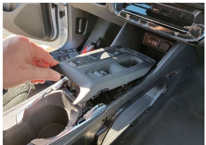
Remove center shifter plate by gently prying from the rear and lifting up. Unplug all harnesses from OEM modules.
