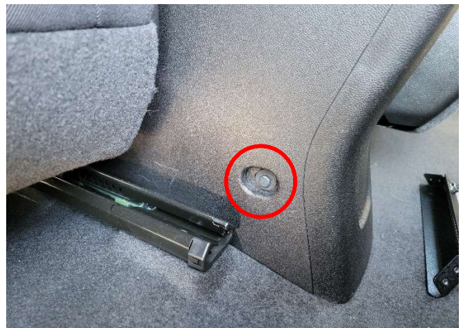
Unbolt the rear 10mm OEM fasteners and set aside.
